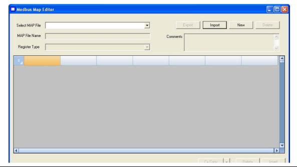
3. To view or edit registers that are contained in an existing MAP file, click on the *Select MAP File* drop-down list and select the appropriate file. The registers will load into the table.
